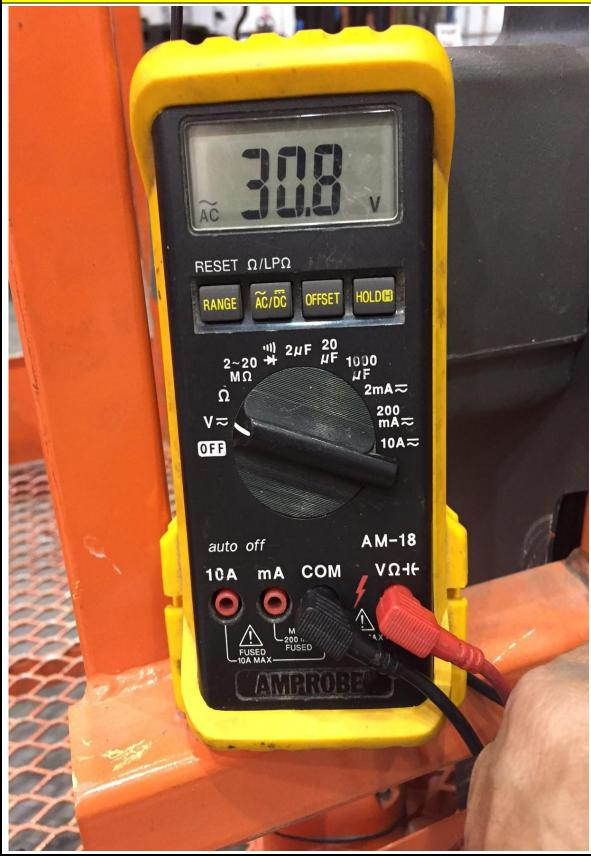
Measurement taken from JLG manlift to earth ground without the Fluke SV225 "Stray Voltage Eliminator" adapter (30.8 VAC / Ghost voltage)
