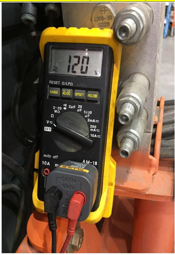
\*Measurement taken from JLG manlift to earth ground with the Fluke SV225 "Stray Voltage Eliminator" adapter (0.167 VAC / True voltage).
